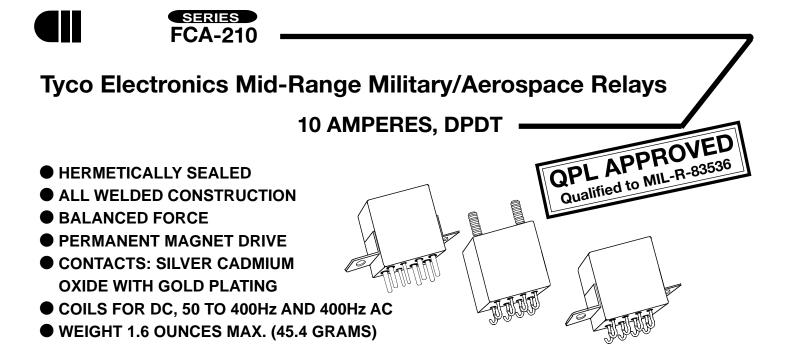
The Series FCA-210 relay is a polarized single-side stable design, where the flux from a permanent magnet provides the armature holding force in the deactivated state, and its flux path is switched and combined with the coil flux in the operated state. This results in appreciably increased contact pressure in both states over that of a spring return nonpolar design. We also manufacture other versions of this relay:
